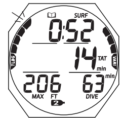
Fig. 33B - LOG DATA 1 (Deco during dive)
