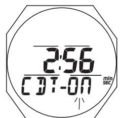
Fig. 106A - CDT STATUS (On, running)
