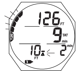
Fig. 74 - DECO ENTRY (during audible)
