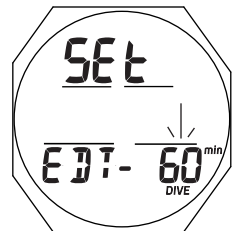
Fig. 42 - SET EDT ALARM
