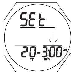
Fig. 50 - SET SAFETY STOP (Time then Depth)
