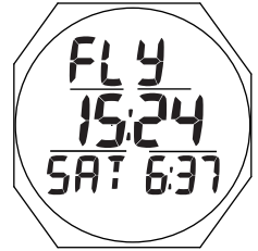
Fig. 28B - FLY/SAT (after a dive)
