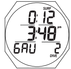
Fig. 94 - GAUG SURF MAIN (after dive # 2)
